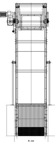
Fabricated parts material: \*Stainless Steel AISI304 / \*Stainless Steel AISI316
