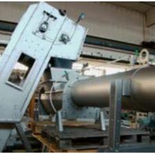
The inlet hopper and the elephant trunk can be easily modified to accommodate the layout needs. The RHW washer compactor is suitable for the following applications.
